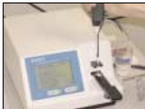
Vapor pressure osmometer ensures all extenders are osmotically balanced
